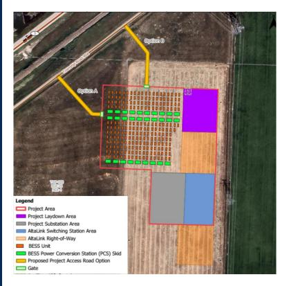
Jumbo BESS is proposed to interconnect to the existing AltaLink transmission line 1037L located approximately 80 metres to the east. Planning, consultation and construction of the transmission line, switching station and structures will be completed by AltaLink.
